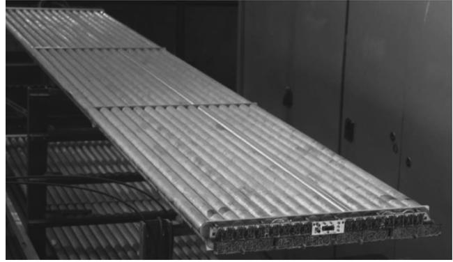
Fig. 37. A block of the muon system at the test-bench. Protective housing is removed.
